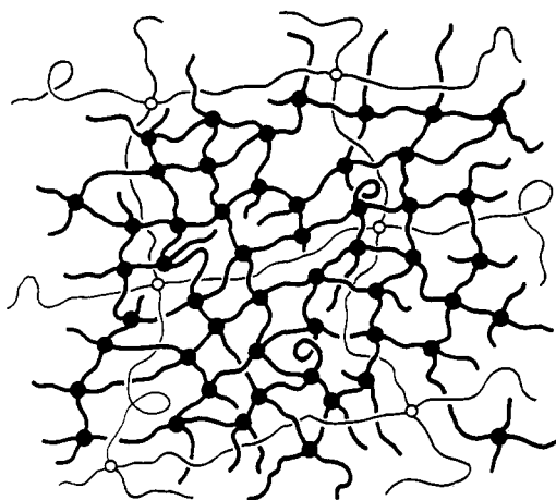
Figure 5. A bimodal interpenetrating network, in which the short-chain cross-links are represented by filled circles and the long-chain ones by open circles.
